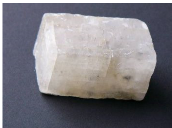
Viking Sunstone found in ship wreckage! Calcite crystals like Icelandic Spar create a double image, splitting light into two rays. If the crystal is held east-west, the double image becomes a single image and thus allows a sailor to locate the sun. The crystal's refractive qualities continue to be useful even in low light, on a cloudy day, or for a while after the sun has set.
